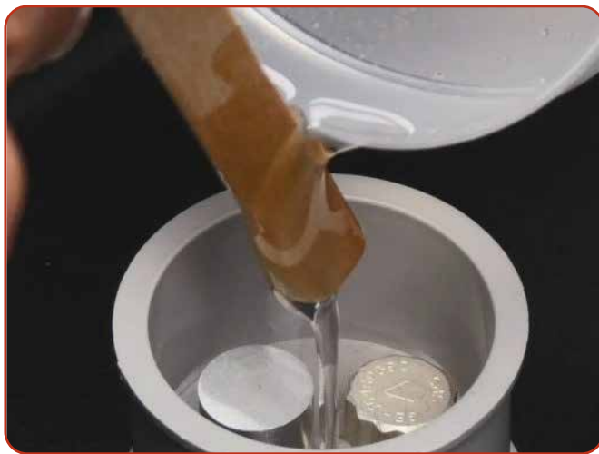
Easy access to directly pour epoxy into mounting cups
